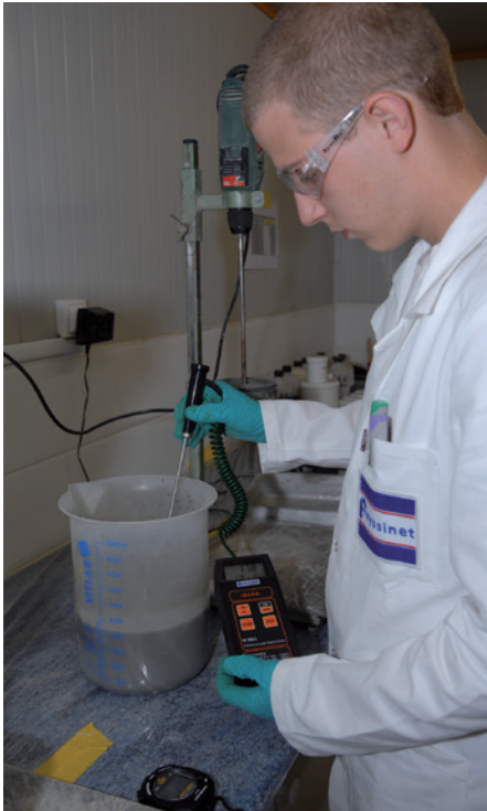
Formulation of cement grout in a Freyssinet laboratory
